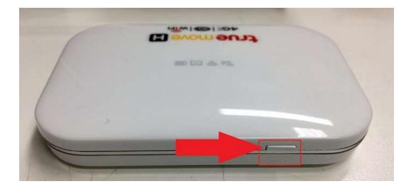
7. Press and hold the button until 4 LEDs are blinking and then
