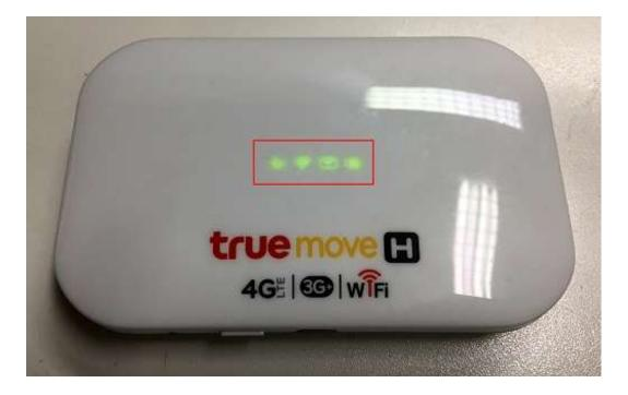
9. Once LED is on, it will be the last one (battery) which means it's starting up and connecting the network
